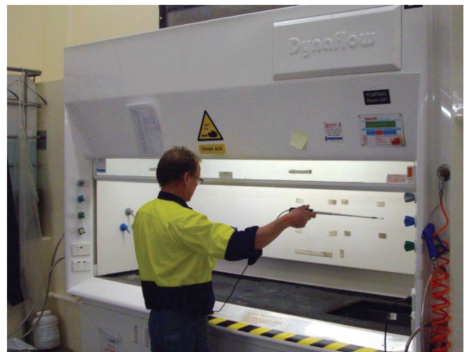
Above: Fully Operational Dynaflow GRP EX fume cupboard custom designed and successfully tested in Australia to withstand an explosive force of 20 grams C-4 explosives.
