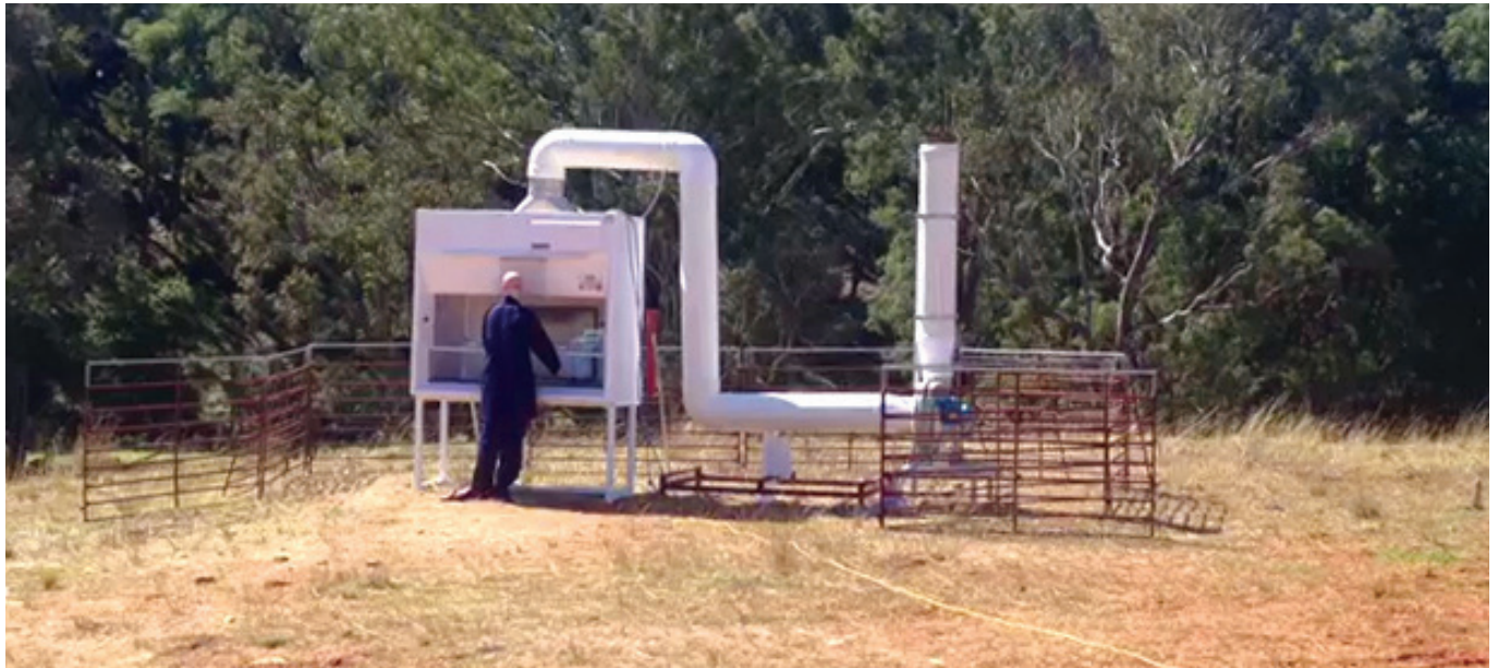
Above: Fully Operational Dynaflow GRP EX fume cupboard custom designed and successfully tested in Australia to withstand an explosive force of 20 grams C-4 explosives.
